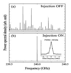
Fig. 11. (a) Multimode structure of a 240-GHz pulse from the UCSB FEL with no injection-locking signal. (b) Single high-power line obtained with injection locking (the insert shows the extremely narrow width of this line). Reprinted, with permission, from [17].
