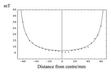
Fig. 3. Variation of the normal *B*-field along a diagonal on the surface of a thin square plate of FB6H heaferrite (see text).
