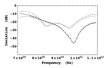
Fig. 5. Predicted isolation (continuous line) and back reflectances (co-polar: long dashed line; cross-polar: short dashed line) for a circulator designed to give optimum performance at 100 GHz. The points are measured isolations.
