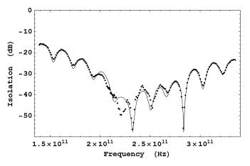
Fig. 7. Isolation of a circulator designed for optimum performance at 240 GHz. The line is the predicted performance and the points are the measured values.
