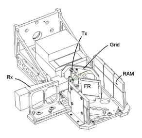
Fig. 13. Feed-module for the compact range (see text).
