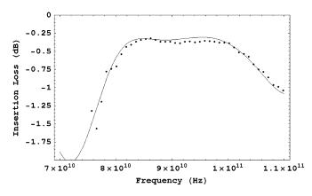
Fig. 6. Predicted insertion loss (line) for a circulator designed to give optimum performance at 100 GHz. The points are measured insertion losses.
