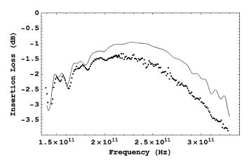
Fig. 8. Insertion loss of a circulator designed for optimum isolation at 240 GHz. The thin line is the predicted performances and the points are the measured values.
