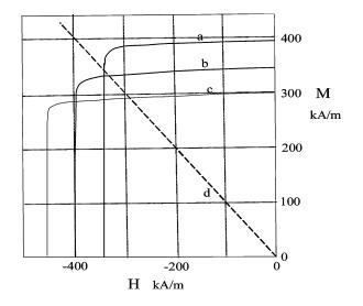
Fig. 2. Near-rectangular demagnetization curves of the FB9H hexaferrite ceramic from TDK,<sup>1</sup> at temperature: (a)  $-40 \,^{\circ}$ C, (b) 20  $^{\circ}$ C, and (c) 100  $^{\circ}$ C (based on the supplier's data sheets). The operating point for a thin plate of a material is at the intersection of the line M = -H (line d) with the demagnetization curve, which is above the knee for FB9H at 20  $^{\circ}$ C and at 100  $^{\circ}$ C, but below the knee at  $-40 \,^{\circ}$ C.
