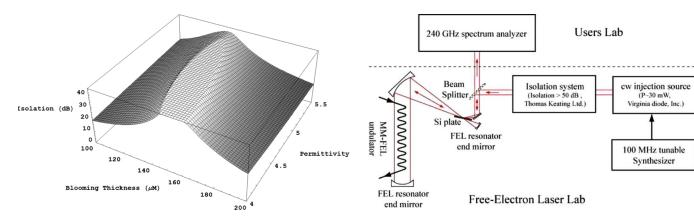
Fig. 9. Predicted isolation of a circulator at 240 GHz as a function of the thickness of the matching (or blooming) layers (in micrometers), and of the relative permittivity of the material of the layer.
