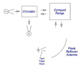
Fig. 12. Schematic of the configuration for the measurement of the 320-GHz monostatic radar cross section of the Planck HFI. The test feed horn is one of many in the focal plane array.
