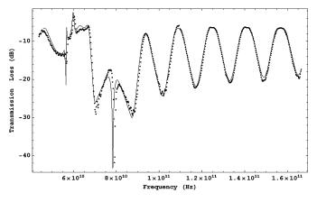
Fig. 4. Co-polar transmittance of a plate of TDK material FB6H, thickness 2.02 mm. The continuous line is the calculated transmittance and the points are measured values.
