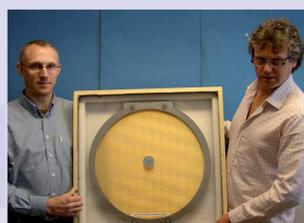
Our photolithographic polarisers are available with a pattern repeat period as small as 2 microns to give excellent polarising efficiency up to 30THz
