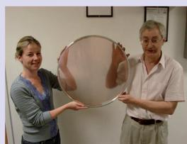
A photolithographic polariser, 500mm in diameter, 10µm pattern period
