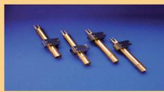
Light-pipe mounted InSb hot-electron bolometers
