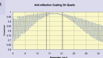
Anti-reflection and reflection coatings can be applied to many materials commonly used in the THz region. The technology is vacuum compatible and has been space qualified.
